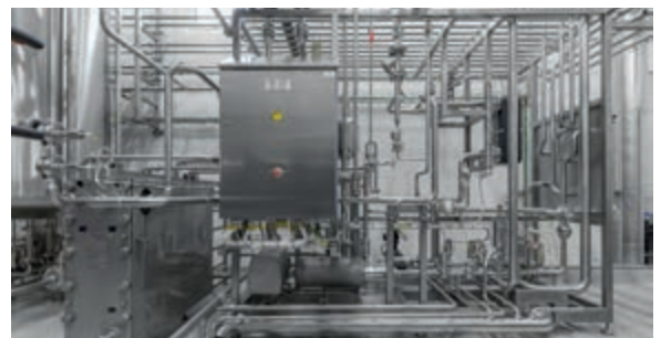
Flash pasteurizer: to ensure quality and shelf life before bottling and to interrupt fermentation for the production of non-alcoholic beverages.
