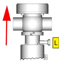
The valve is opened in direction 'X' by means of control air, and is closed from top to bottom by means of spring power without any leakage. Different media fed from the tank or the piping system are separated in a leakage-free fashion by means of two, independently acting valve discs with double seal function. Any leaks occurring due to damaged valve plate seals are drained to the exterior without pressure via the leakage discharge (L).
