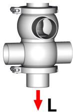
The valve opens from the top down by means of control air and closes bottom to top by means of spring tension without loss of product. In the closed setting, mix-proof separation of the media flowing in the upper and lower valve chambers is ensured by two independently closed valve plates. Any leaks occurring due to damaged valve plate seals are drained to the exterior without pressure via the leakage discharge (L).
