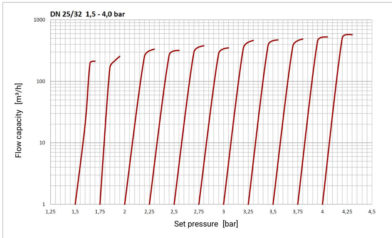
Bunging valve DN15/25 | DN25/32 | DN40/50 Set pressure: 1,50 - 4,00 bar bar (air 20°C)
