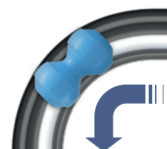
Pigging of DIN bends without product mixing
